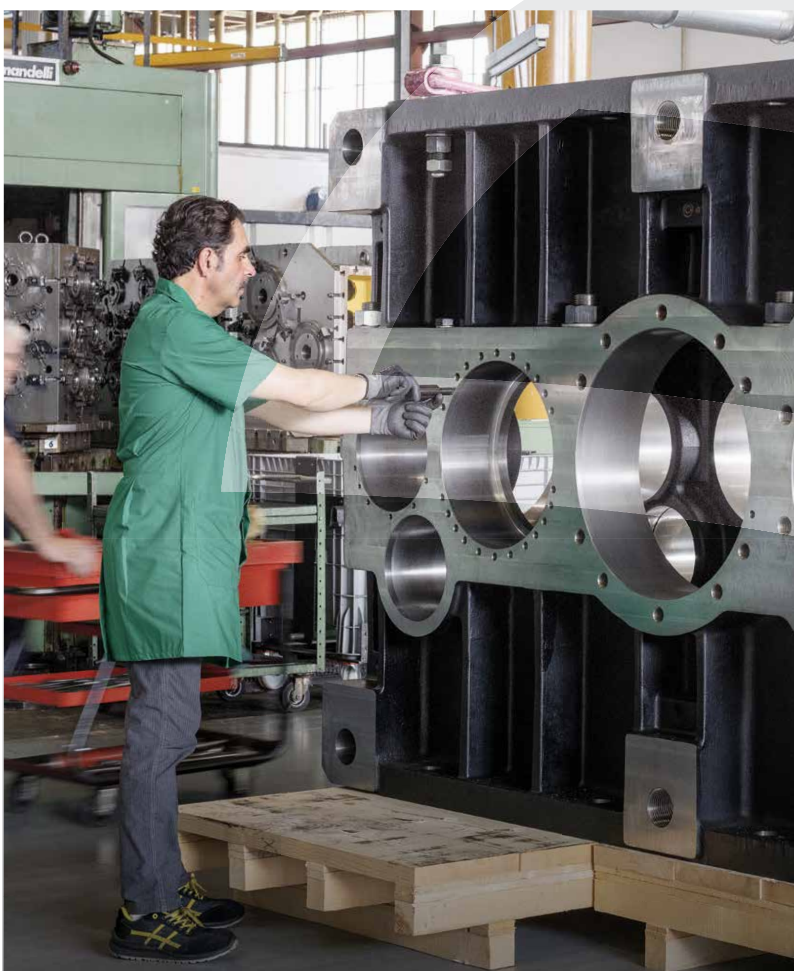
Dedicated area for extra-large housings equipped with boring, milling and 3D control system.
